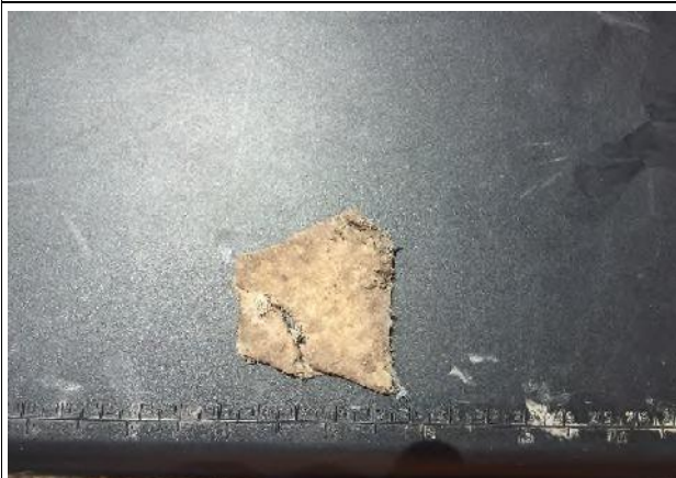
Photograph 27: Bonded ACM fragment observed in surface soils adjacent East of the former quarry/landfill fence line
