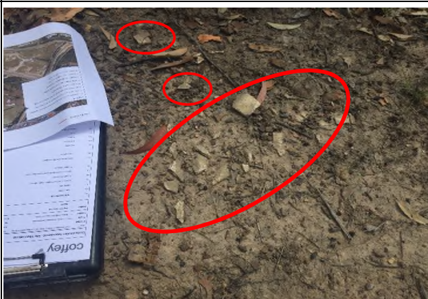
Photograph 28: Asbestos Fragments in site surface soil located in 250m 2 Grid adjacent East of the former quarry/landfill fence line
