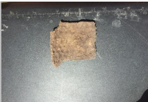
Photograph 25: Bonded ACM fragment observed in surface soils adjacent East of the former quarry/landfill fence line
