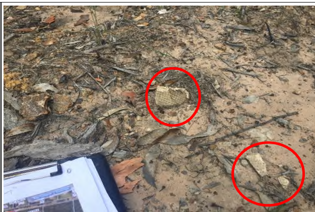
Photograph 26: Cluster of bonded ACM fragments within surface soils.
